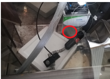
Fig. 1: „Installation position“ in the WB workspace; red: external monitoring of the real ambient temperature (see exempl. Fig. 2)
