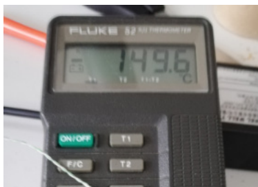
Fig. 2: Real ambient conditions of the valve in the WB workspace Temperature measurement
